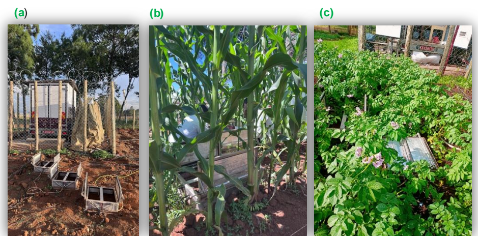
(a) Experimental set-up with the 3 chambers per plot and the trailer that houses the gas analyzers, (b) maize plot, (c) potato plot
